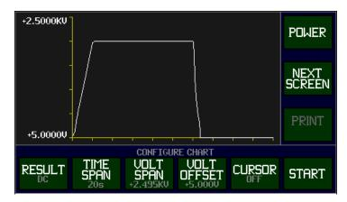
The 4700 can collect DC and AC measurement results over a user configurable time span. Starting data collection can be performed either manually or automatically. The measurement results are configured on the Primary Measurement Results Screen.
