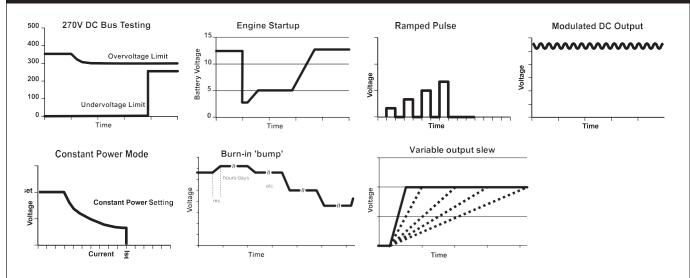
SGX model provides constant power mode allowing independent setting of the max voltage, current and power
