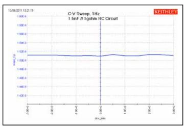
Figure 14. Results of measuring parallel RC combination of 1.5nF capacitor and  $1G\Omega$  resistor. This graph is from the *VLF\_1nF\_1gohm* UTM (*vlfcv\_measure\_dual\_sweep\_bias\_fixed\_range* user module).
