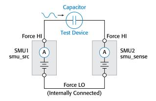
**SMU1 with preamp:** Outputs DCV with superimposed ACV and measures AC voltage. SMU2 with preamp: Measures AC current at OV DC.
