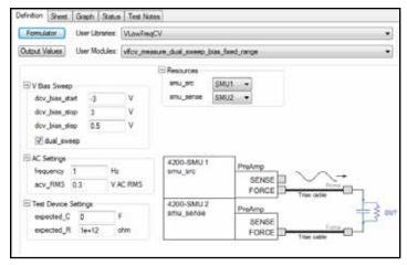
Figure 3. UTM GUI view of the definition tab of vlfcv\_measure\_dual\_sweep\_bias\_fixed\_range user module.
