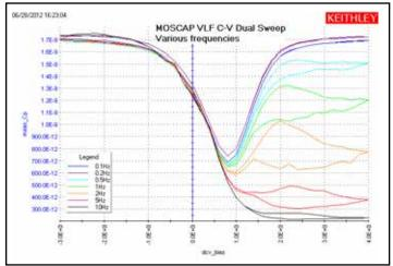
Figure 11. A VLF C-V sweep of a MOScap at various frequences from 100mHz to 10Hz created using the VLF\_CV\_Examples project. This graph is from the VLF\_moscap\_Vsweep UTM (vlfcv\_measure\_sweep\_bias\_fixed\_range user module).
