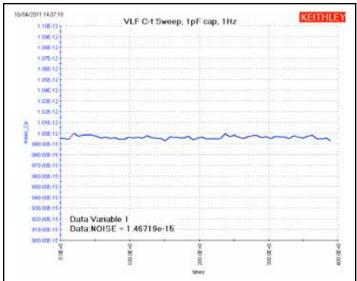
Figure 10. Results of C-t measurements of nominal 1pF reference capacitor, using VLF capacitance technique at a test frequency of 1Hz. This graph is from the VLF\_cap\_time UTM (user module vlfcv\_measure\_sweep\_time).
