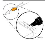
Universal IC Cap Use this cap to prevent shorting the probe tip between IC pins.
