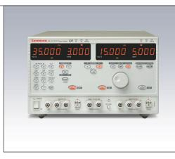
setting is very fast requiring only three key presses to set to 5 volts, for example, (V, 5, OK). To set a more precise level such as 12.725 volts requires more key presses, but can still be done in seconds.
