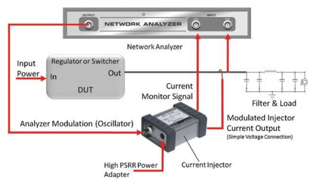
The J2112A Current Injector supports non-invasive phase margin measurements. You can actually use it to measure the stability of your power supplies WITHOUT having to break the control loop. Simply connect the Current Injector output (+ and - leads) to the signal of interest and you can measure the impedance, stability, or step load response.
